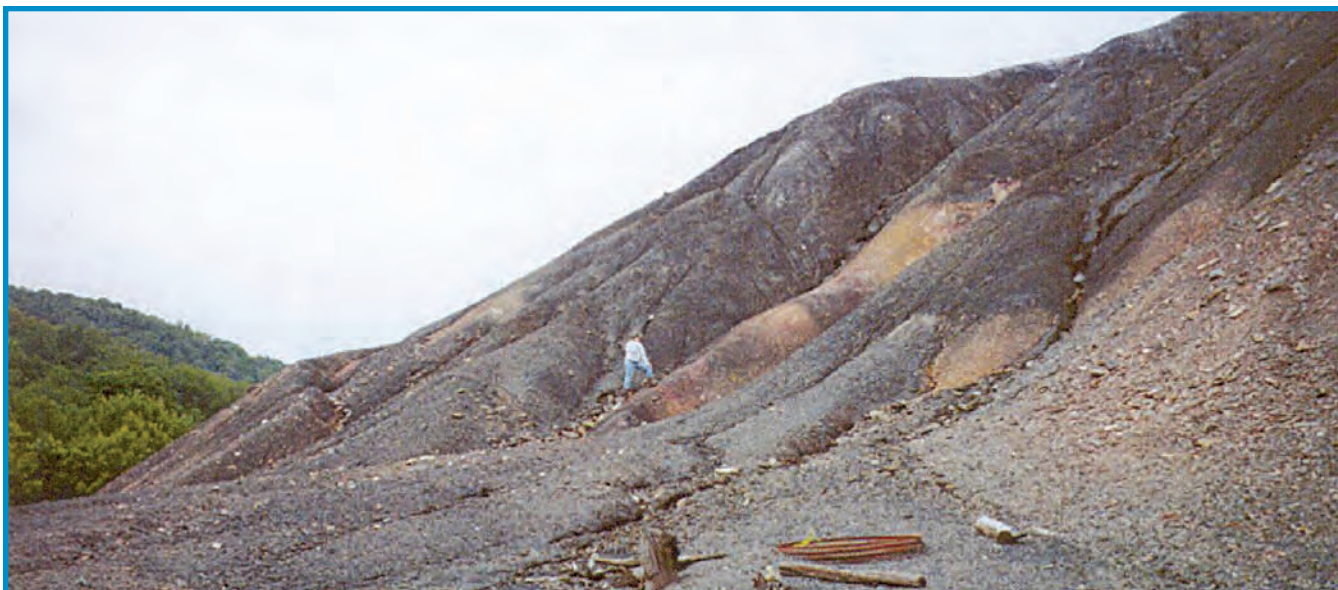
Figure 2. Unightly mountains of low-grade coal and rocks, some as tall as 300 feet and thousands of feet long, are the fuel source for Seward Station. Boney piles are a major source of acid runoff into rivers and streams. (Reliant Energy)
