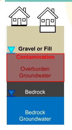
Must have soil-like material present between the bottom of the building foundation and contaminated groundwater to use VISLs.
