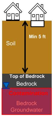
If a vapor source is only in bedrock groundwater, measure to the top of the bedrock.
