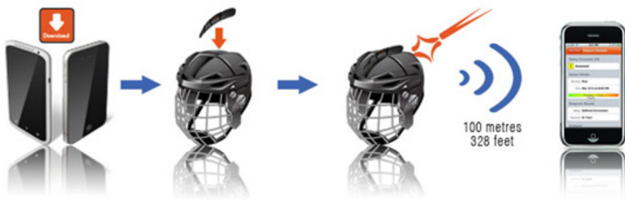
Figure 4. Helmet accelerometers and wireless data system used in a recent study of linear and rotational head accelerations in youth ice hockey players.
