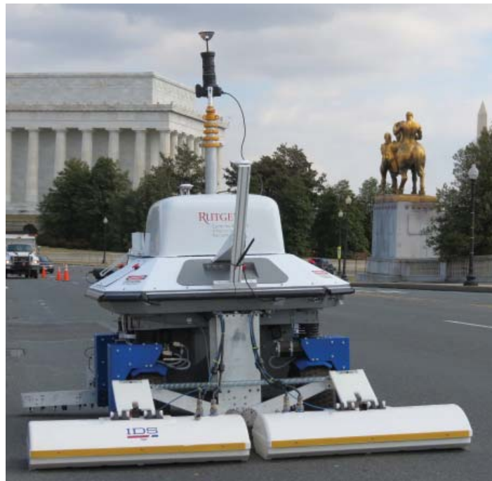
The RABITTM – a robotic system for condition assessment of concrete bridge decks, in operation on the Arlington Memorial Bridge in Washington, DC (Photo courtesy of Dr. Nenad Gucunski, Rutgers University)
