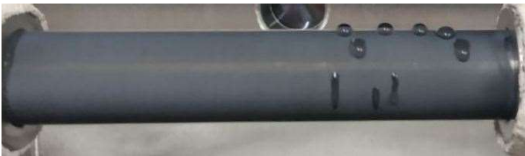
Figure 13: Film Wise Condensation left and Drop Wise Condensation right (Budhathoki, 2023)
