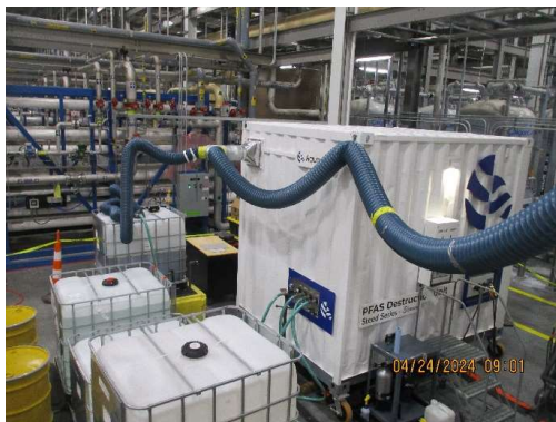
Figure 3. Commercial-scale HALT reactor operating at a water quality building during a 2-week pilot trial (April, 2024) and PFD showing sampling points.
