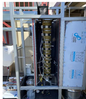
Figure 2. Process flow diagram (PFD) and picture of small-scale HALT reactor used for Development Work.
