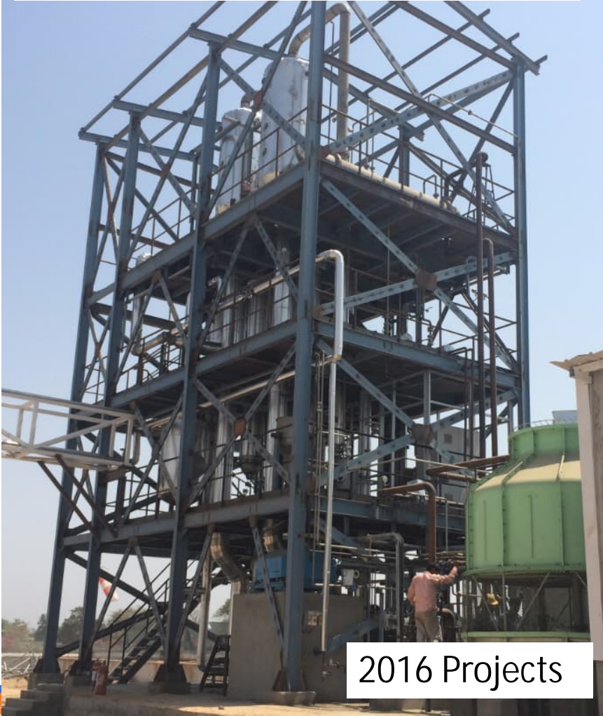
Multiple Effect Evaporator 1x100%
