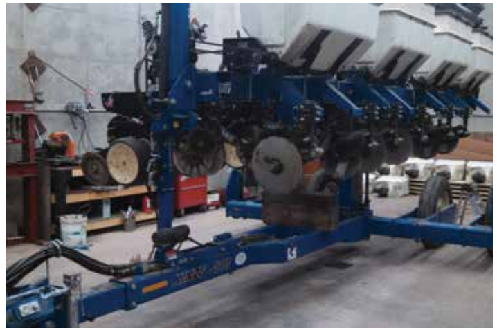
Figure 2: Kinze seeder folded for transportation and storage
