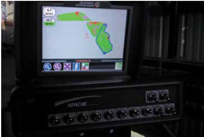
Figure 4: Apache Sprayer, showing view during operation and summary screen after spraying. Red indicates zones of overspraying and purple indicates zones of underspraying, largely speed related.
