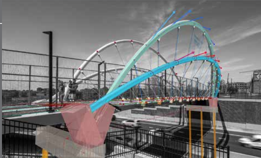
Parametric Model Juxtapositioned with Completed Bridge
