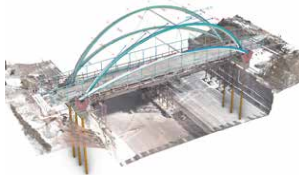
Parametric Model Juxtapositioned with Surveyed Bridge Prior to Completion
