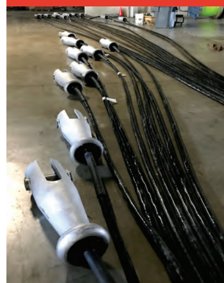
Figure 2: Custom terminations with synthetic support pennants
