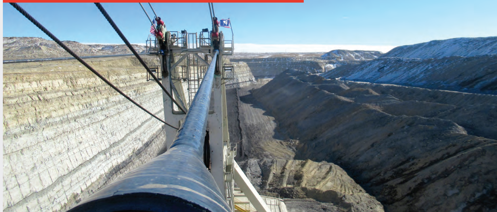
Figure 3: High strength synthetic pennants in a fatigue sensitive environment
