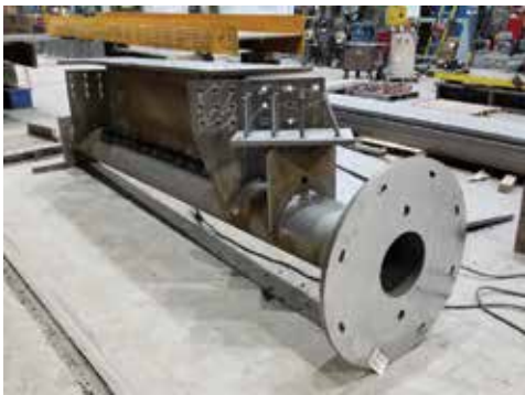
Cable anchor assembly in the shop
